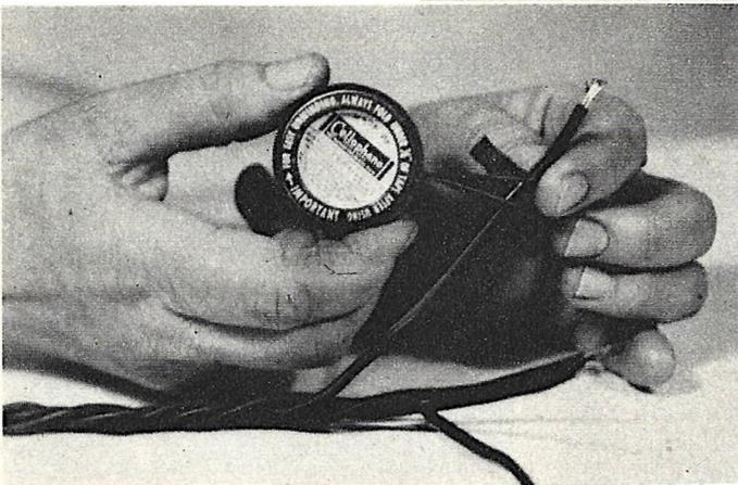
**A**BOVE — Colored tape wrapped around plug-in coils serves two useful purposes—holding the windings in place and identifying the frequency band of the coil. Each coil should be marked with a different color. Left—Small strips of colored tape can be used to good advantage as code markers for a group of wires, such as a battery or power supply cable. Each wire should be given a separate color or combination of colors.
