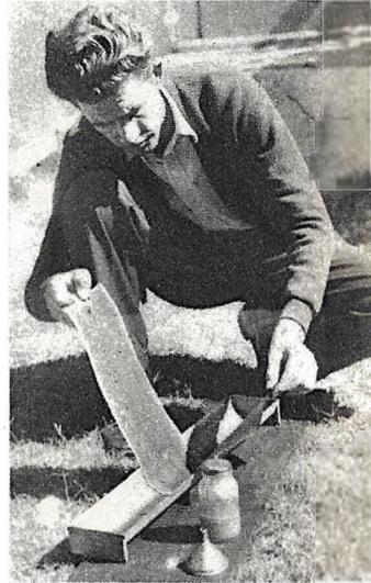
Right—Washing the completed record of the thermograph in a solution of alcohol and shellac to give it permanent protection against damage.
