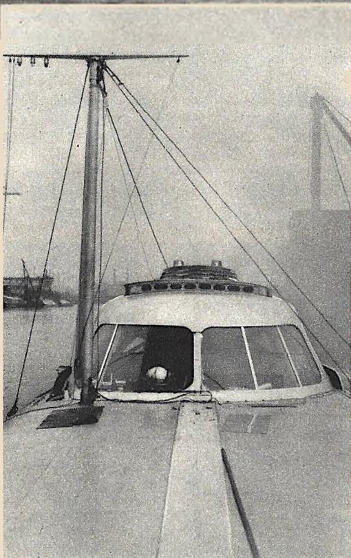
The off-center mast is collapsible. The roof of the pilot house raises 6 inches for ventilation. Note smokestack louvers designed to create upward air currents to carry off engine smoke. All exhausts are through this stack.
