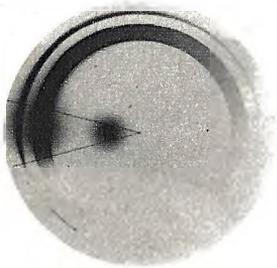
sity of the flashbulb output, and a third arc, made by two holes showing direction of rotation. Note broad peak of lamp output as indicated by dense region. The synchronizer is a trifle early in its operation, but still well on the peak. Left: Record of foil-filled lamp (small size), at 1/200 second. Note narrower peak as compared to record of wire-filled bulb.
