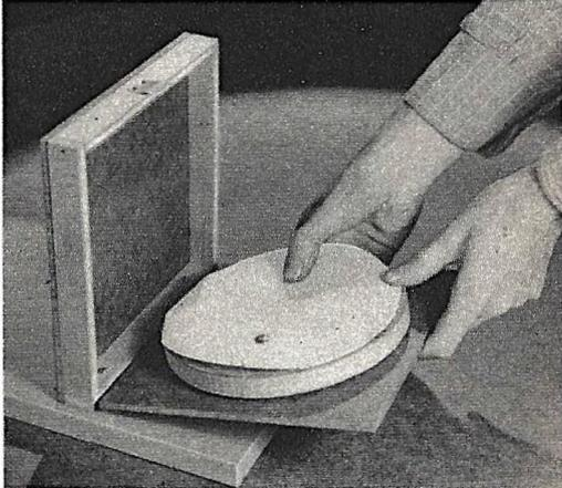
Thumbtacking a bromide paper record sheet to the wooden disc preparatory to making a test. This is done in the dark-room, by a suitable safelight lamp.
